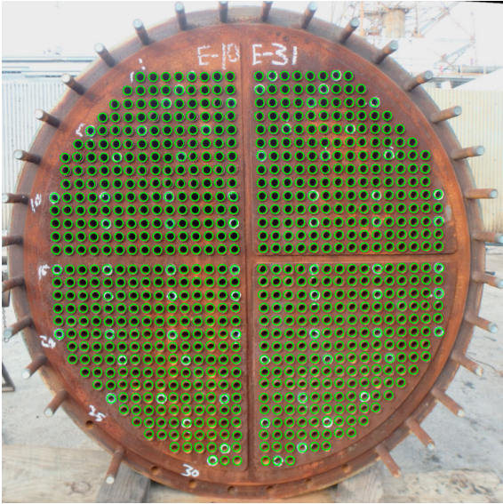
Figure 1: Result of the automatic photo detection feature using a photo taken onsite of a shell and tube heat exchanger.
